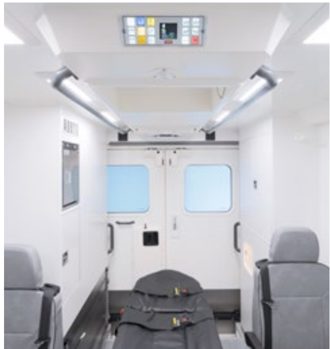
The ceiling centre is used to contain medical equipment, energy and oxygen supply as well as the central panel used to control the ambulance table and further essential functions.
