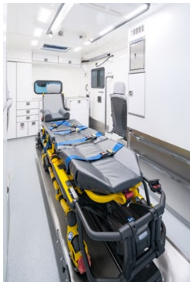
Three attendant seats in the patient compartment - all with integrated three-point seat belts, seat indicator and seat heater (option) - enable a comfortable treatment of the patient.
