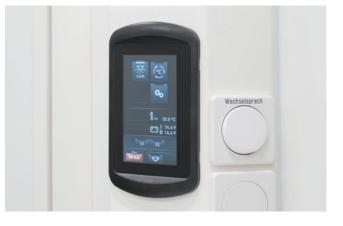
Many central functions such as lighting or air conditioning and heating systems can be controlled via the touch panel in the patient compartment.
