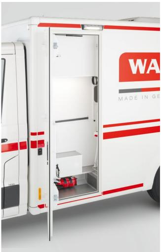
Scoop stretchers, CombiCarrier and other equipment can be easily stored outside of the patient compartment.
