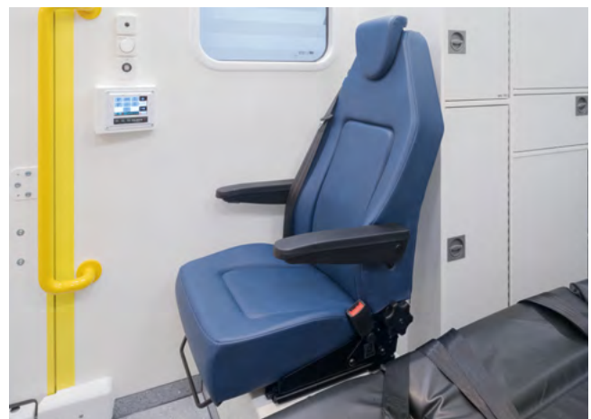
Comfortable seat with integrated three-point belt, 2 arm rests and adjustable back and head rests.
