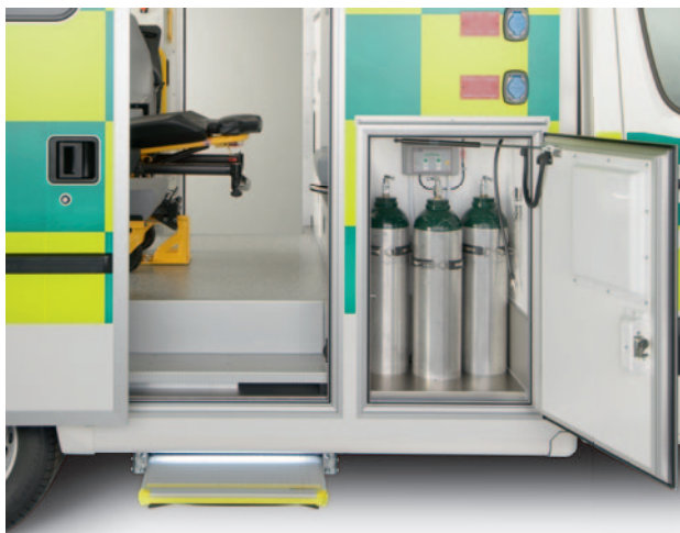
Oxygen cylinders are easily accessible from the outside.
