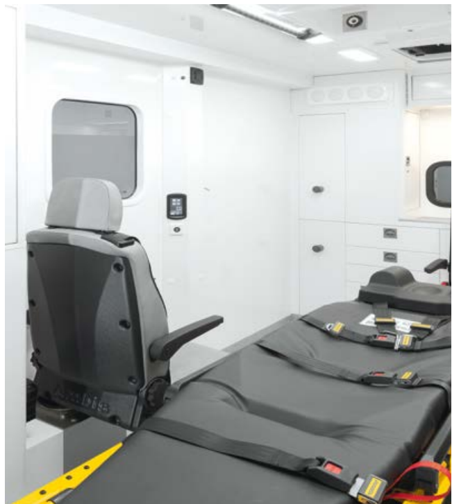
The touchpanel on the left hand side allows the attendant to control all of the main functionalities while sitting, which leads to a much higher safety for the attendant during operation.
