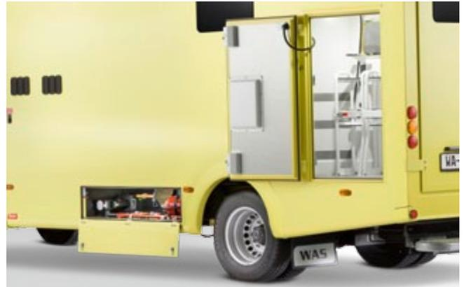
Compact and secure: Oxygen supply in the exterior storage compartment, rescue tools in the under-floor compartment.
