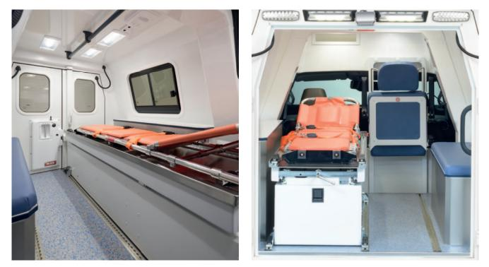
The right-hand and the left-hand side walls are equipped with large storage compartments. Robust air line rails in the floor fix the stretcher support or even material to be transported. The attendant seat is retractable to have an optimum use of space.
