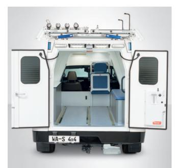
After removing the stretcher support, in just a few simple steps, the spacious interior can be loaded with material.
