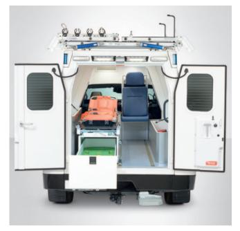
Integrated heavy-duty drawer for the accommodation of scoop, spine board or rescue tools.
