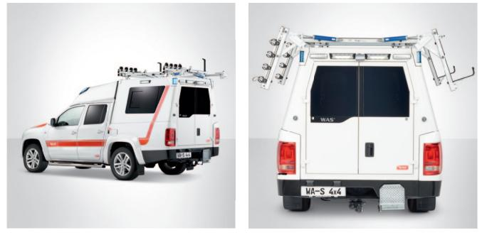
With the swing-away frame structure, material can be easily loaded from either the right or the left side of the vehicle.
