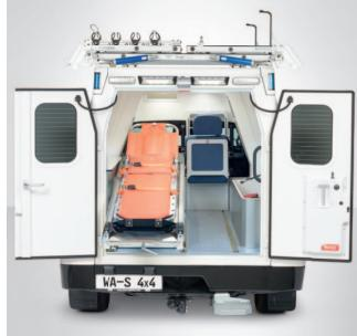
The stretcher support is swung down to a lower loading level, to ensure the safer loading of the patient.
