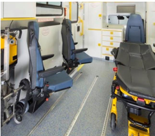
Two fully tested forward facing attendant seats incl. integrated three-point seatbelts, this allows also a 45° seat position of the paramedic in driving direction.
