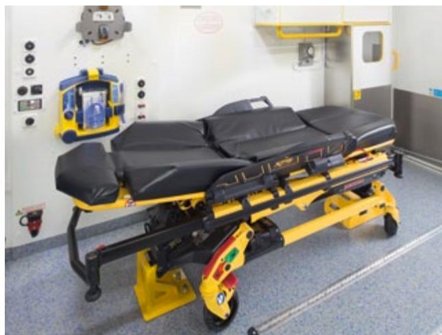
Airline rails in the floor facilitate multiple options for mounting a standard or a bariatric stretcher.
