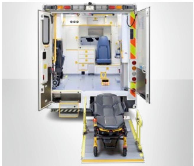
The new designed patient lift has a capacity of 500kg and facilitates an ergonomic loading and unloading of the stretcher. It features a fully automatic bridge plate and internally housed manual operation facility.
