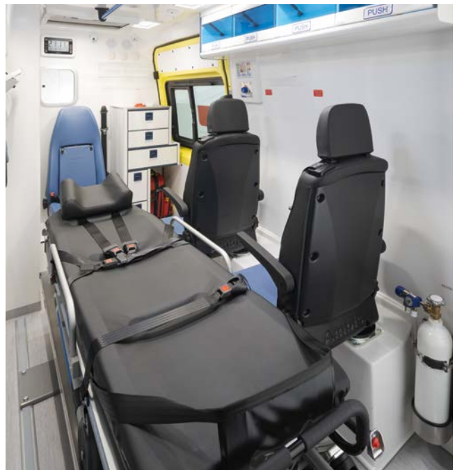
Two foldable seats on the right side for paramedics or family members.
