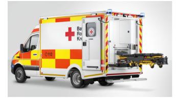
The Stryker Powerload stretcher system incl. the Power Pro XT stretcher facilitates the loading and unloading of heavy patients.
