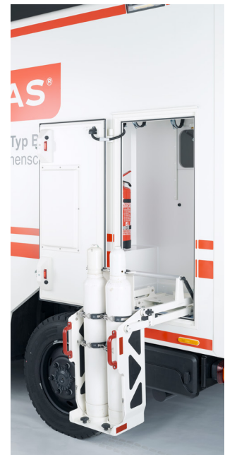
Lifting supports for ergonomic removal of the second stretcher and oxygen cylinders.
