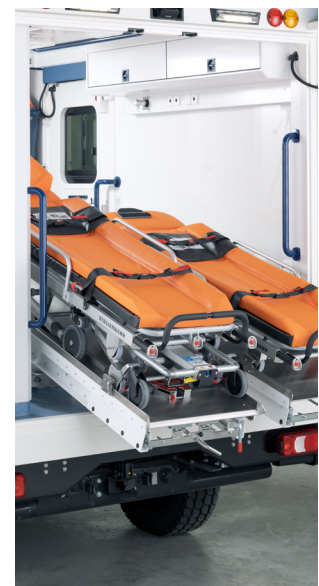
Lifting supports for ergonomic removal of the second stretcher and oxygen cylinders.
