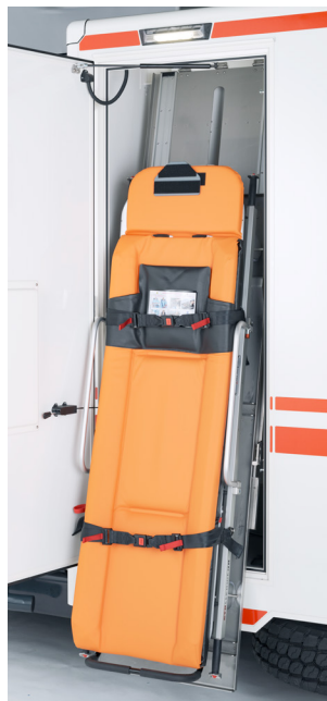
Lifting supports for ergonomic removal of the second stretcher and oxygen cylinders.
