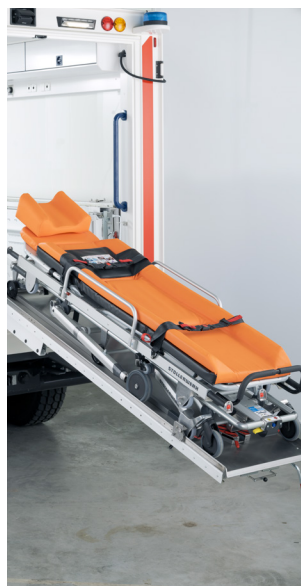
Lifting supports for ergonomic removal of the second stretcher and oxygen cylinders.
