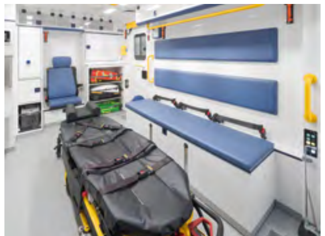
Place for further attendants on the right side. Storage space is below the seat.
