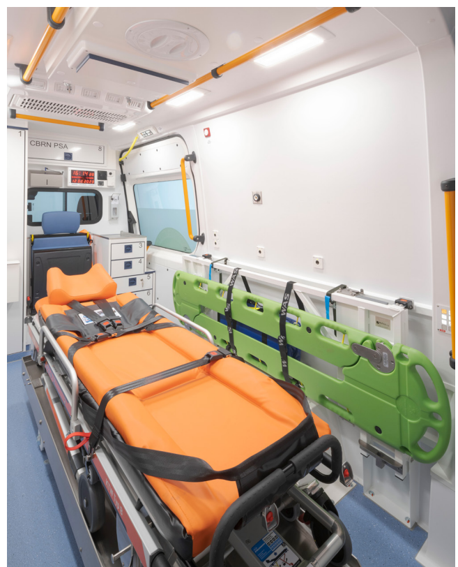
The second stretcher support with a holder for scoop stretcher and accessories is attached to the side wall.
