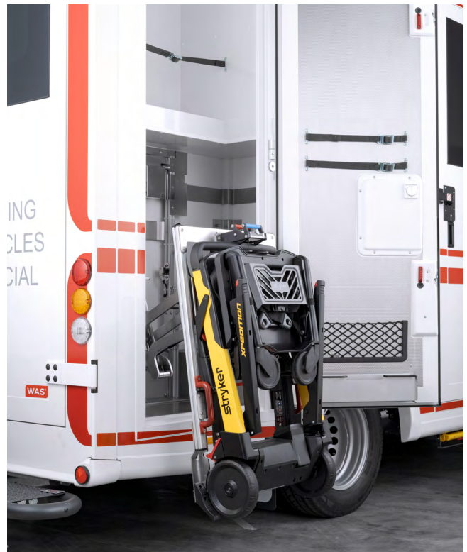
WAS Lift Assist: Ergonomic loading and unloading of the carrying chair at the push of a button – flexible use with different loading heights.
