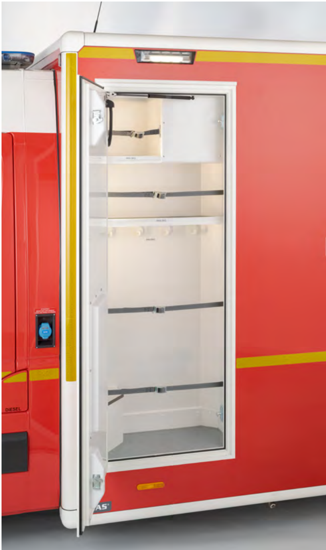
Large exterior storage compartment with integrated lighting and rear safety lights.
