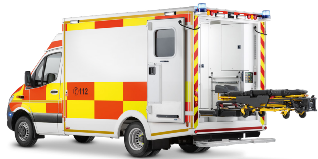
The Stryker Powerload stretcher system incl. the Power Pro XT stretcher facilitates the loading and unloading of heavy patients.
