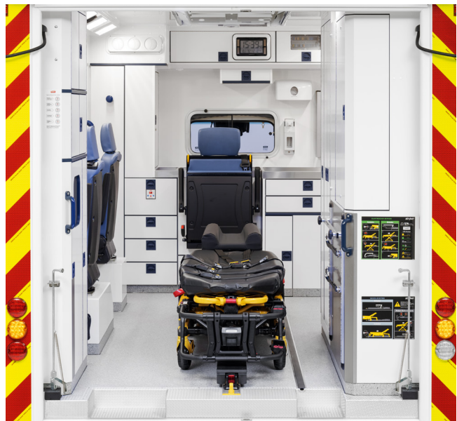
An airline track system is integrated into the floor for the loading of medical equipment and gear.
