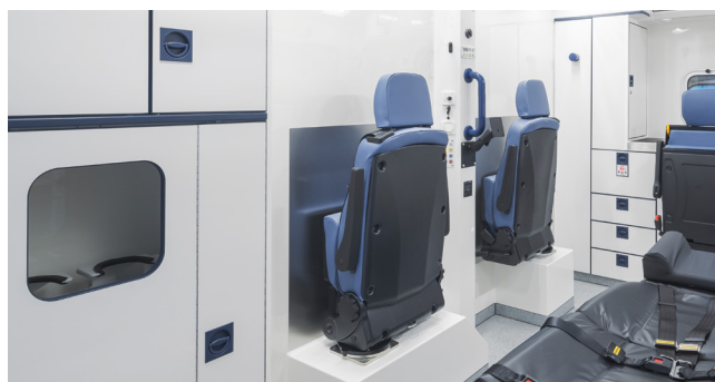
Three attendant's seats in the treatment area – all with integrated three-point belts – enable ideal patient care.
