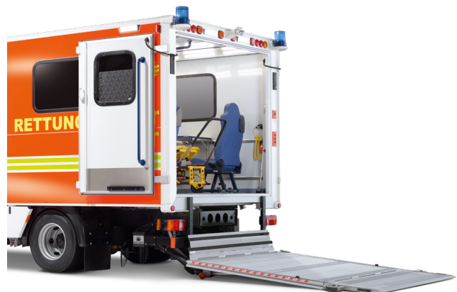
The electronic loading ramp can be lowered completely to ground level, making it easier to load and unload the vehicle safely.
