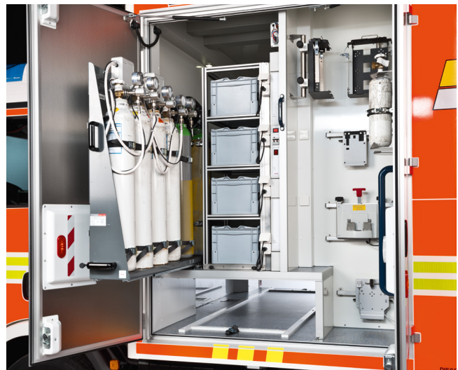
Oxygen and compressed gas supply are easily accessible on a heavy-duty pull-out.
