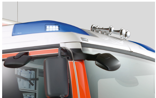
The warning system is equipped with energy-saving LED technology.
