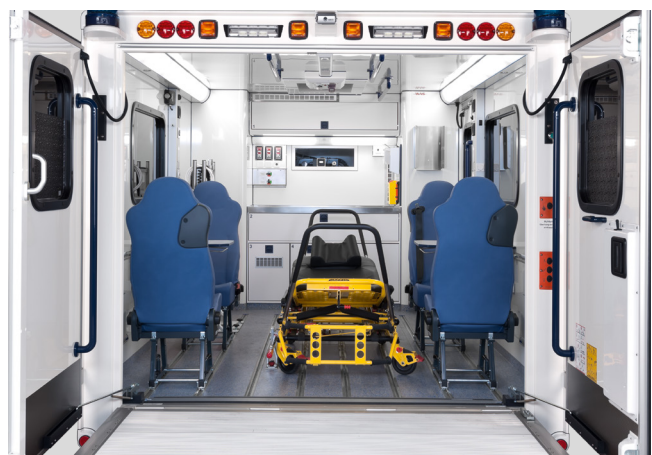
Up to four seats and two tables can be securely attached to the airline rails and easily removed
